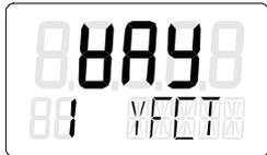
2. Use the
