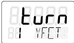
3. Call the "2.YAGL" parameter. To do this, briefly press the
