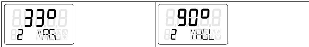
3. Check whether the value displayed of the "2.YAGL" parameter matches with the setting of the transmission ratio selector. If required, change the setting of the transmission ratio selector to 33° or 90°.
