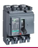
Circuit breaker basic frame, ComPact NSX160H, 70kA at 415VAC 50/60 Hz, 160A, without trip unit, 3 poles
