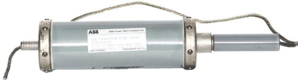
The COL fuse is a full range current-limiting capacitor fuse designed for outdoor use only. COL fuses exist in voltage classes of 2.8 kV, 5.5 kV, 8.3 kV, 15.5 kV and 23 kV and are applied to individual capacitor units in outdoor stacking equipment. The COL fuse is current-limiting, indicating and disconnecting.
