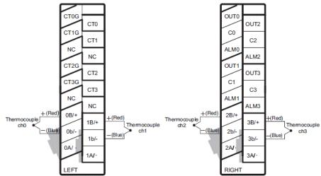
\* Colors in parentheses () are the wiring colors (color of Y terminal) for thermocouples made by Keyence Corporation. In the case of a non-contact thermocouple, these become + (yellow) and - (red).
