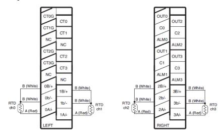
\* Colors in parentheses ( ) are the wiring colors (color of Y terminal) for RTDs made by Keyence Corporation.
