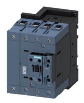
power contactor, AC-3, 65 A, 30 kW / 400 V, 4-pole, 20-33 V AC/DC, 50/60 Hz, with integrated varistor, main contacts: 2 NO + 2 NC, auxiliary contacts: 1 NO + 1 NC, screw terminal, size: S3
