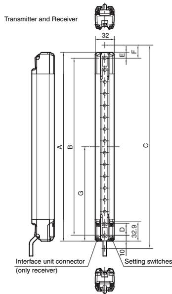
If the length for a single GL-R unit is 1280 mm or greater, use the following antivibration mounting bracket additionally as an intermediate support bracket. The antivibration mounting bracket must be selected according to the mounting bracket and installed on the center of the GL-R unit indicated as position "G".
