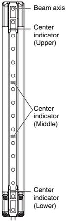
Center indicator (Upper) : indicates whether interruption is present in the top beam axis or not. (clear or blocked)
