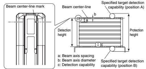
**Detection zone :** The zone in which the specified target detection capability can be detected. The detection zone of the GL-R indicates a square area formed with the detection height and the operating distance. When an object of the specified target detection capability is present in this area, the light of the GL-R is blocked, and then the OSSD goes to OFF state.
