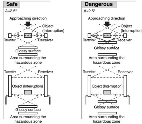
When determining a specific installation distance, refer to the following values including the installation tolerance.
