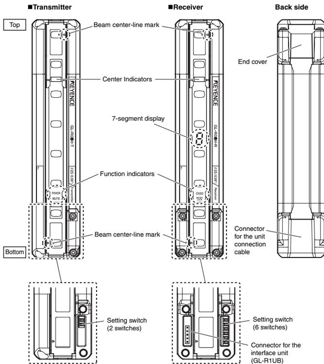
\* The side where the end cover has already been installed at shipment is the top side.
