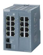
SCALANCE XB216 managed Layer 2 IE switch, 16X 10/100 Mbit/s RJ45 ports, 1x console port, diagnostics LED red redundant power supply; IEC 62443-4-2 certified; temperature range 0 to +60 °C DIN-rail mounting; default EtherNet/IP.
